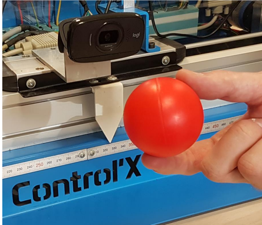
Target tracking by image analysis under Simulink
